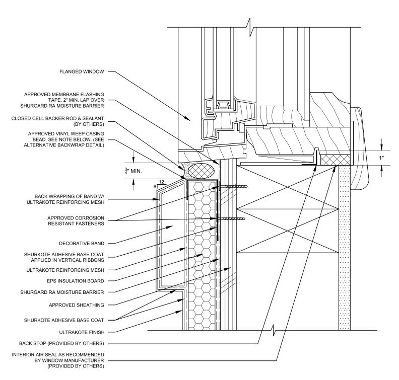
NOTE: AT HORIZONTAL WALL SURFACES, INCLUDING LEDGES, CAPS, SILLS, ETC., A MINIMUM SLOPE OF 6 INCHES IN 12 INCHES IS REQUIRED
